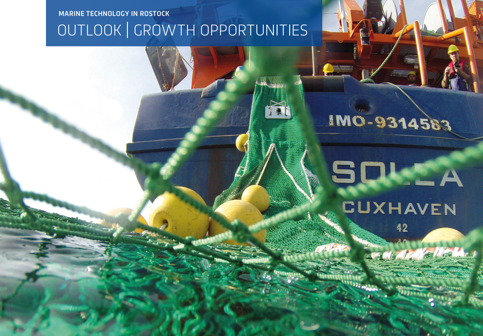
the fisheries research vessel „Solea“ testing selective trawls
